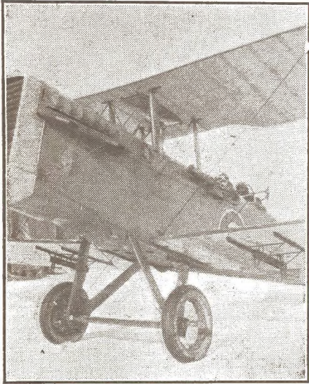
Here's real detail for our modelers—the nose of the British D.H.9, offering unusual opportunity to study motor exhaust, center-section struts, and the Vickers gun mounting outside the pilot's pit. Those racks on the wing carried 112-lb. bombs.
