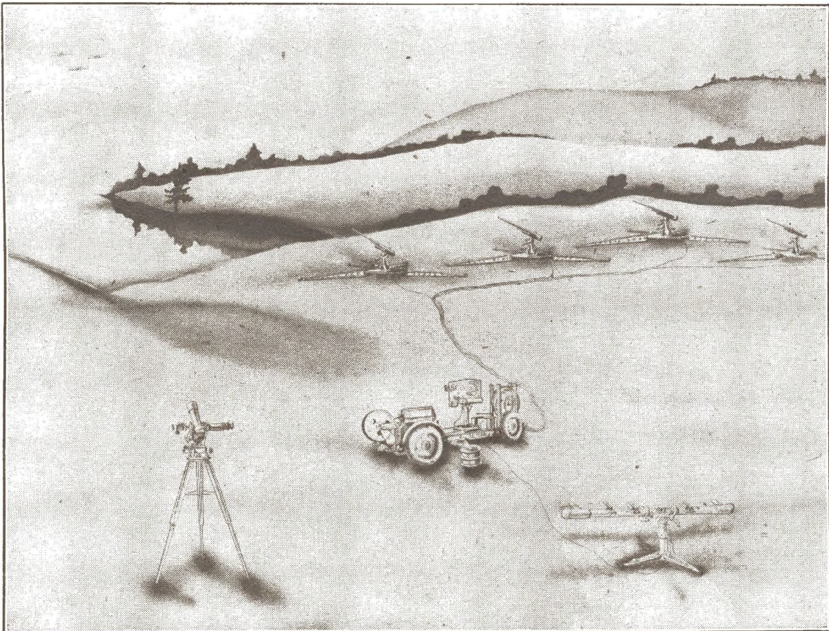
Put them all together and this is what they spell—a complete anti-aircraft battery. In the left foreground is the Tracking Telescope, in the right foreground the Stereoscopic Height Finder, in the center the Automatic Data Computer, and ranged in a semi-circle in the background are the guns. The electric power lines connecting the units inter-relate the action. In the upper left-hand corner of the diagram, raiding planes may be seen approaching.
